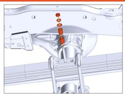
Reinstall the factory U-bolt saddle and install the supplied **Center Pin Spacers** with the correct size flat washer, split washer, and factory center pin nut.
