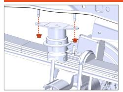
Unbolt factory bumpstop using a 15MM socket.
