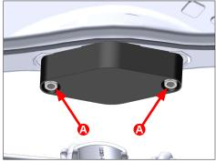
A Torque the coupling nuts to **35 FT. LB.**Repeat for passenger side.
