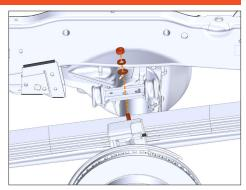
Reinstall the factory U-bolt saddle with correct size flat washer, split washer, and center pin nut.
