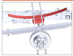
Spray the factory center pin nuts and axle U-bolt nuts with penetrating oil.
