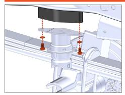
Use the supplied M10 bolts, with flat washers, to attach the bump stop to the bump stop spacer.
