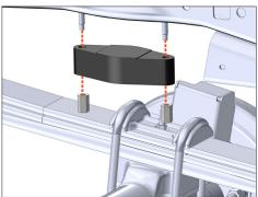
Install the aluminum bump stop spacer using the provided hex coupling nuts.
