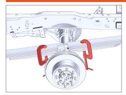
If your factory center pin was damaged, then you will replace it with the supplied shorter replacement pin.
